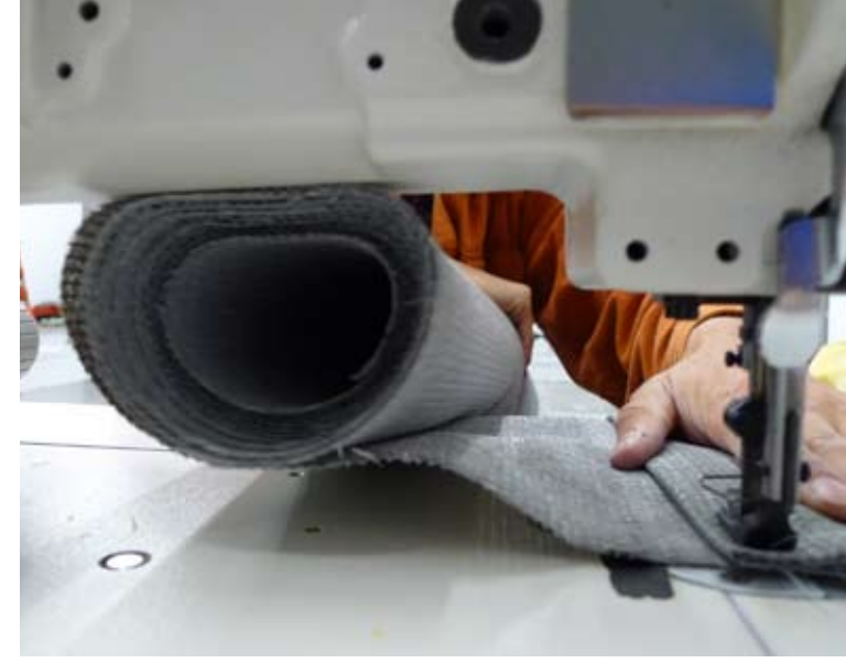
Sewing the roof-membrane
