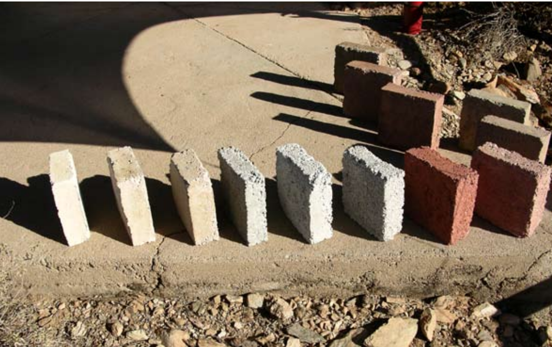
13 test bricks of rammed-earth, 8"x 8"x 3"
