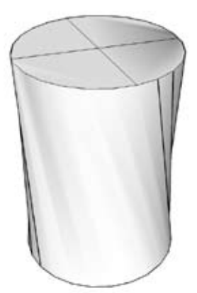
Twisting of a cylinder to produce a hyperboloid
